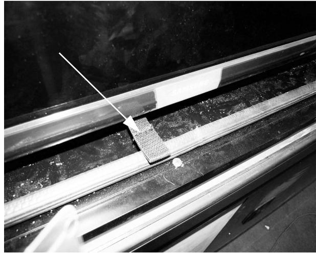
To adjust the TV, pull the black strap (located on back side of TV) straight down to release the TV from the mounting bracket.
