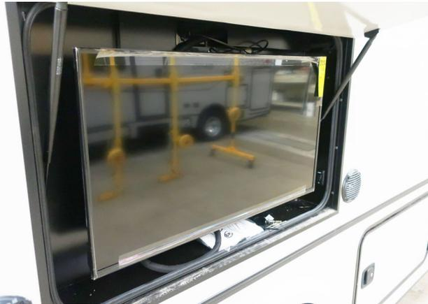
Example of TV located on passenger side lift up panel.
