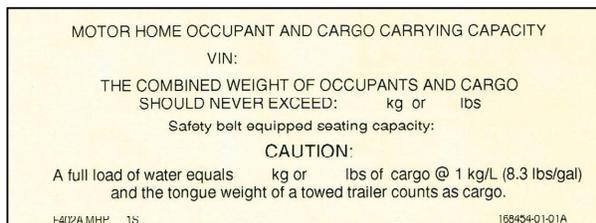
If any weight exceeding 45.4 kg (100 lbs.) is added to your motorhome between final vehicle certification and first retail sale, the occupant and cargo carrying capacity must be corrected and a label similar to the one shown in the following photo will be affixed inside your motorhome.
