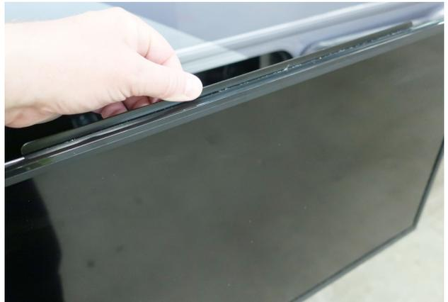
When folding the TV back down press on the metal bracket above-
