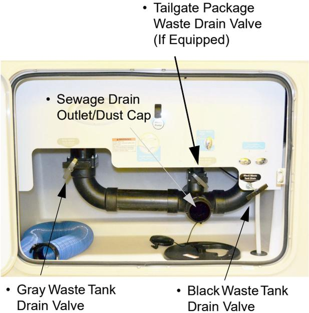
Holding Tank Drain Valves
