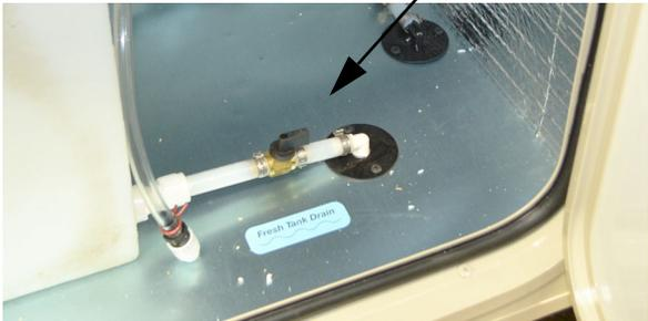
Waterline and Water Tank Drain Valves
