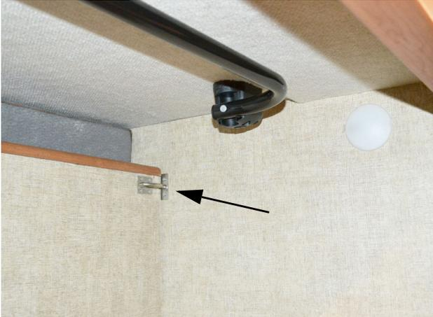
*NOTE: Ensure that security lock (located on front bunk cabinet wall) is fully engaged.*
