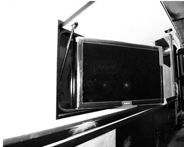
Pull the TV out and pivot to desired position. To return to storage, rotate TV back to center position and press straight back. You will hear a “click” when the TV is secured into locked position.
