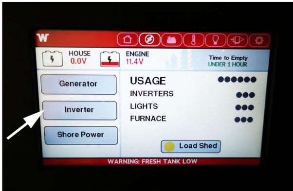
From the main menu select the battery section and the screen with the inverter button will show in the menu.
