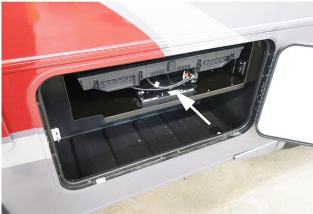
Press lever to the left and the TV will slide out. Then pull up on the top of the TV to secure in the up position.
