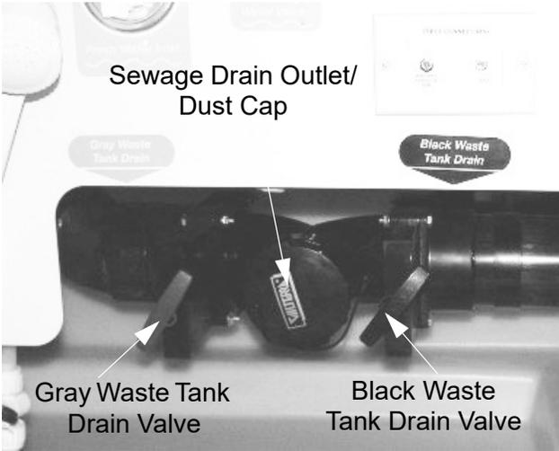
Holding Tank Drain Valves
