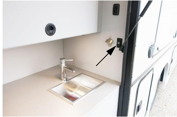
Tailgate Sink Drain Pump Switch
