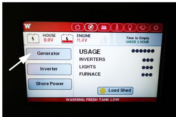
From the main menu select the electrical section and the screen with the generator button will show in the menu.
