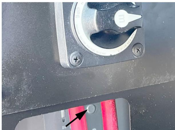
Ensure that the inverter box power button is pushed in for the monitor panel to be able to operate the inverter.
