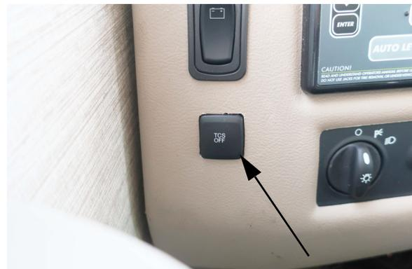
Traction Control Button is located on the driver side left of the headlight switch
