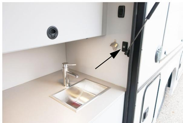
**Sink Drain Pump Switch
