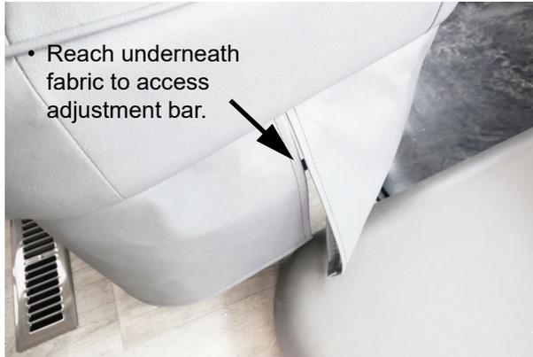
The Driver and the Passenger seats both have an adjustment bar under the fabric in the front. Pull up to slide the seat forward or rearward.
