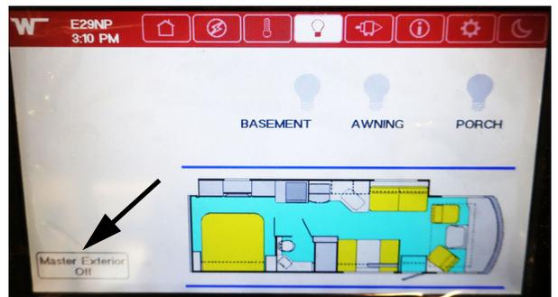
Pressing the Exterior Lights button will reveal the buttons that control the awning, porch, and basement lights. (The basement light command must be turned on for the basement lighting to be powered).
